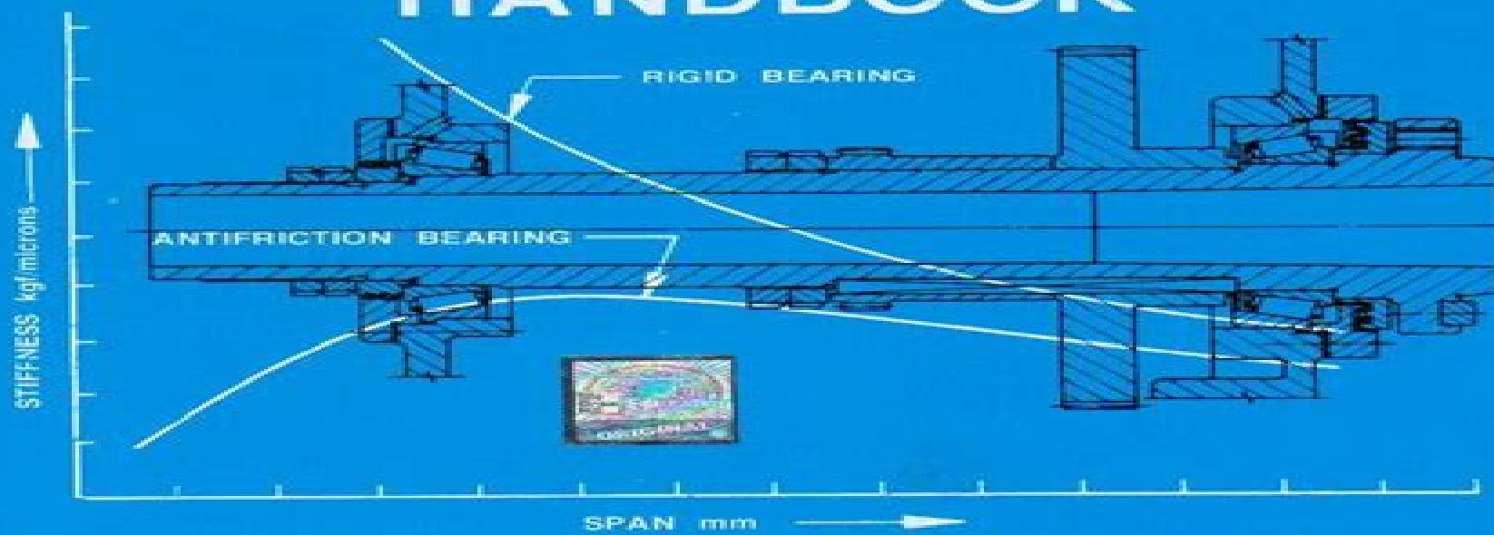
$$S = \frac{P}{\delta_1 + \delta_2} = \left\{ \frac{a^3}{3EI_L} \left[ \frac{L}{\sigma} + \frac{I_L}{L} \right] + \frac{1}{S_A} \left[ \left( 1 + \frac{a}{L} \right)^2 + \left( \frac{a}{L} \right)^2 \frac{S_A}{S} \right] \right\}^{-1}$$
