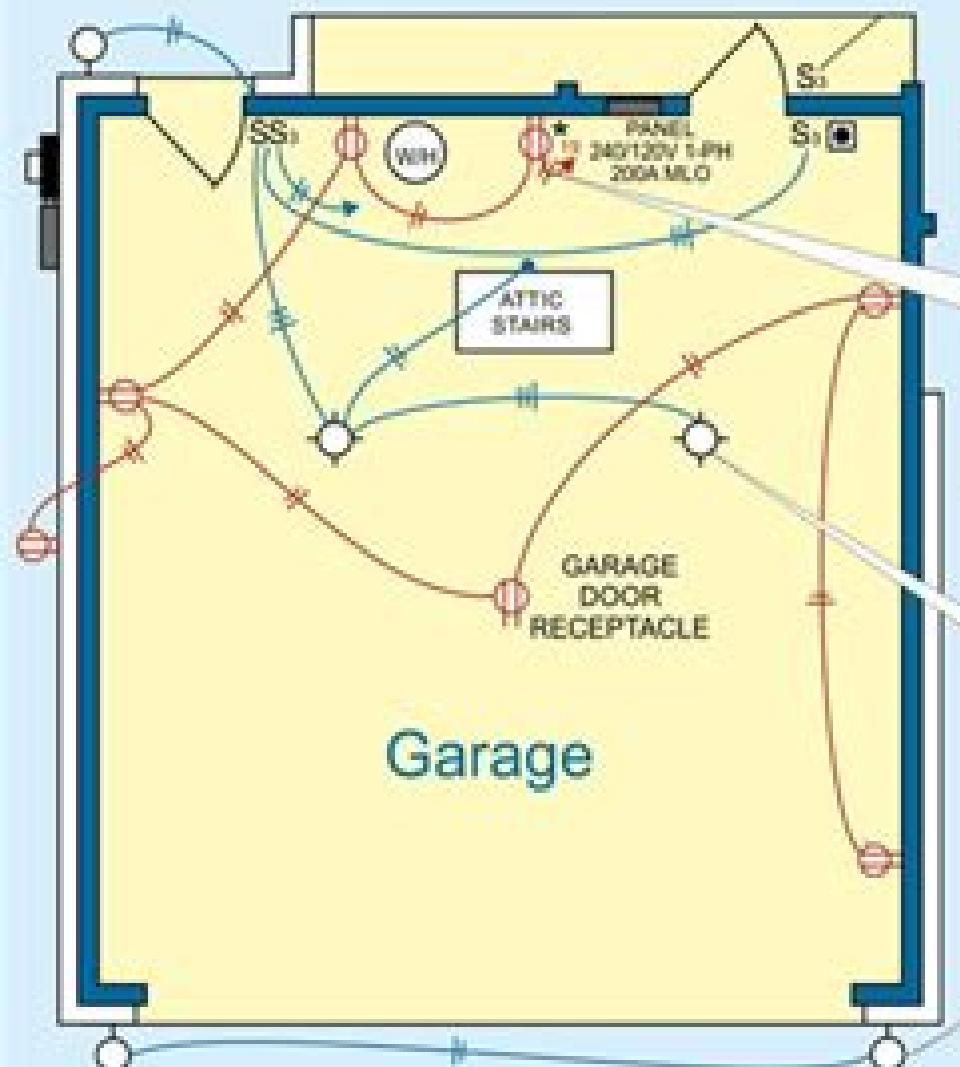
At least one 20A, 120V branch circuit is required to supply the receptacle outlet(s) in attached and detached garages with electric power.
