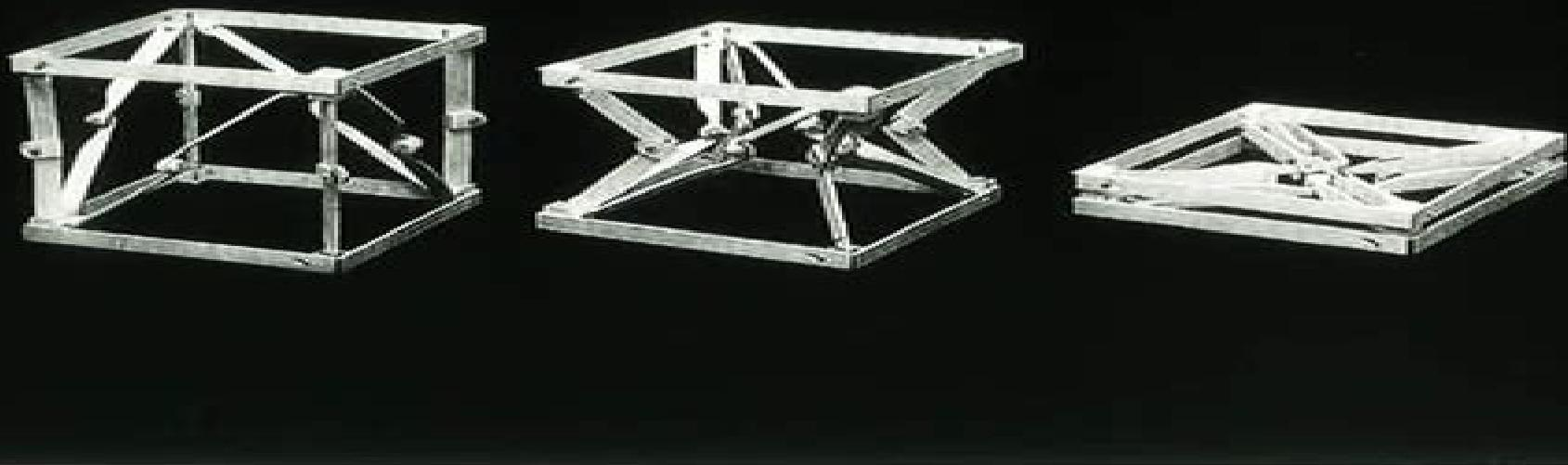
**Fig. 3.** Deployment sequence of NASA STAC-BEAM geometry model.
