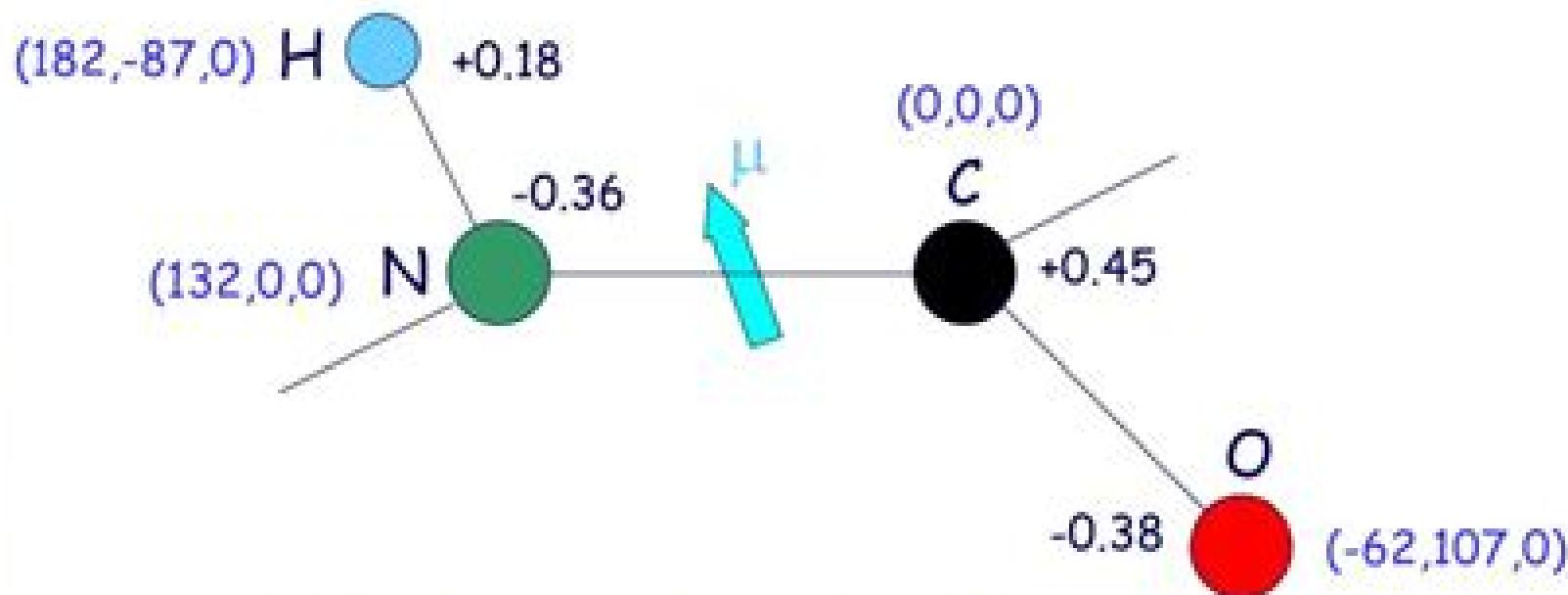
$$\begin{aligned}\mu_x &= (-0.36e) \times (132 \text{ pm}) + (0.45e) \times (0 \text{ pm}) \\ &\quad +(0.18e) \times (182 \text{ pm}) + (-0.38e) \times (-62 \text{ pm}) \\ &= 8.8e \text{ pm} \\ &= 8.8 \times (1.602 \times 10^{-19} \text{ C}) \times (10^{-12} \text{ m}) \\ &= 1.4 \times 10^{-30} \text{ C m} = 0.42 \text{ D}\end{aligned}$$
