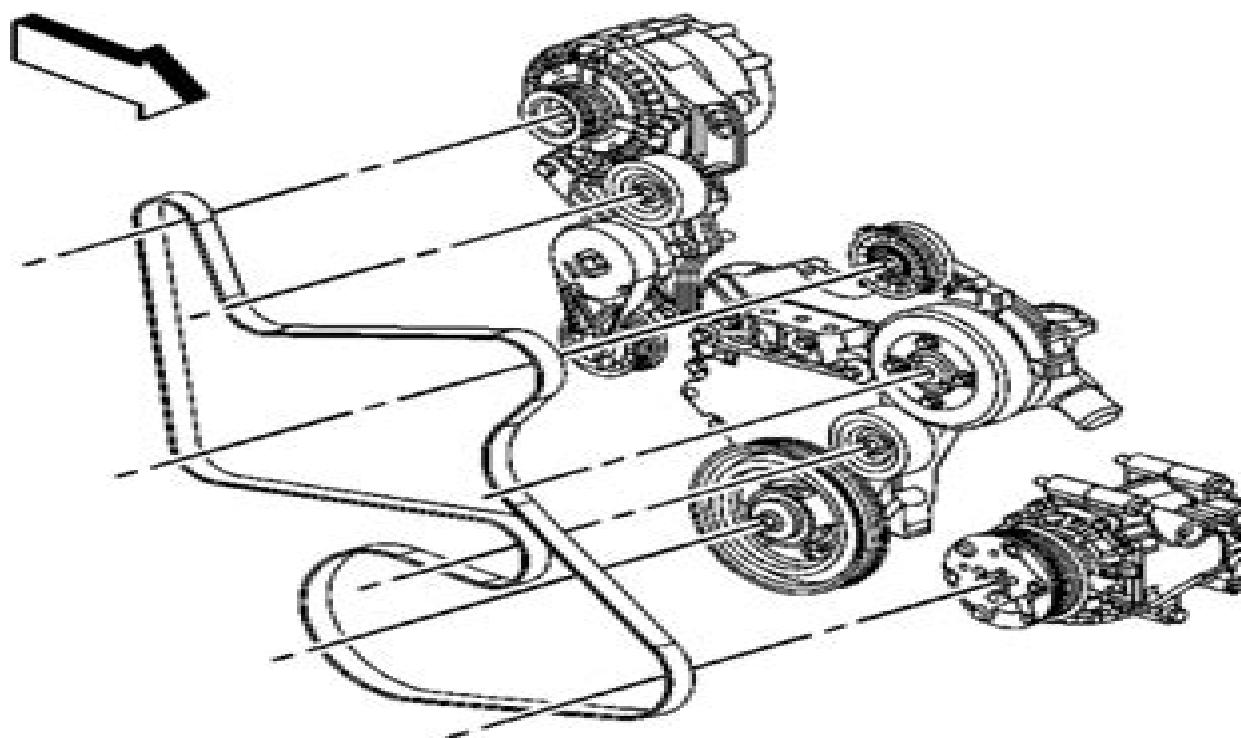
**Fig. 12: Removing/Installing Drive Belt**
