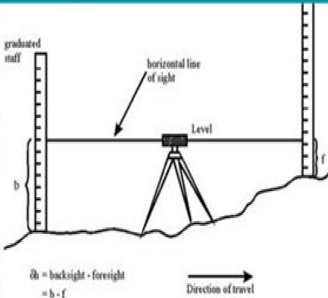
$$\begin{aligned} dh &= \text{backsight} - \text{foresight} \\ &= b - f \end{aligned}$$
