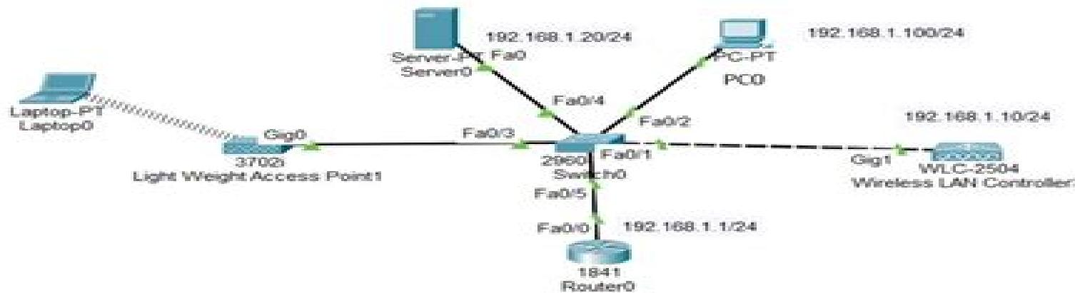
2. Click on the Wireless LAN Controller icon and go to the **Config** tab. Click on the **Management** interface and set the management IP address to **192.168.1.10**, subnet mask to **255.255.255.0**, and default gateway to **192.168.1.1**. Submit a screenshot of these settings.
