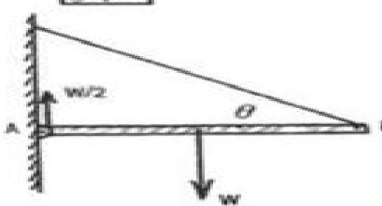
4. Consider the boom supported by hinge A and by a cable B. Vectors are shown for the weight  $W$  of the boom at its center, and  $W/2$  for vertical component of upward force supplied by the hinge.
