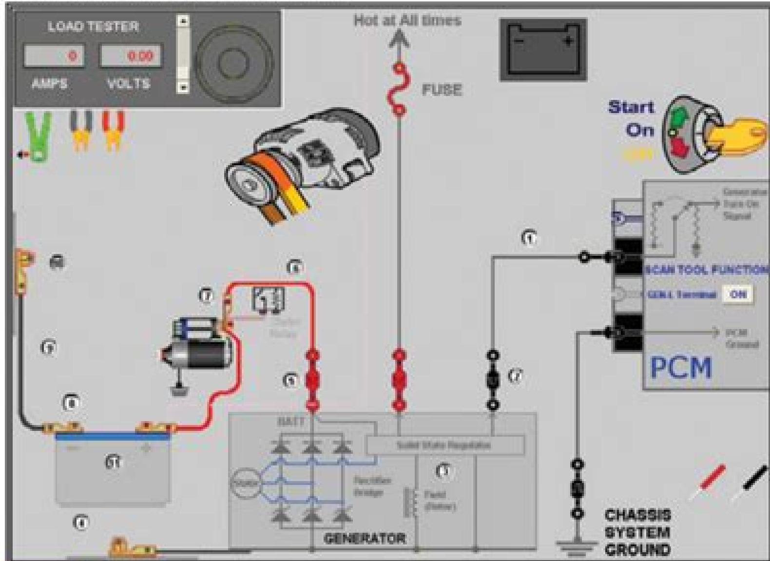
A fault has been inserted into the Charger circuit. Using the meter to troubleshoot the circuit, find and identify the fault.
