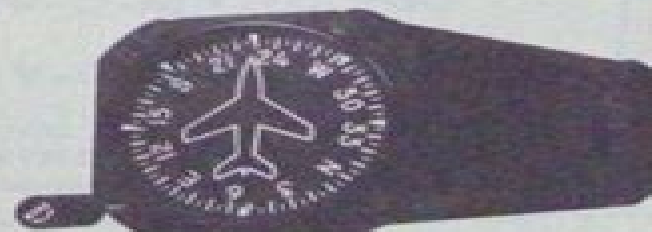
DIRECTIONAL GYRO NAV-O-MATIC 300 PART NO. 30370-0100
