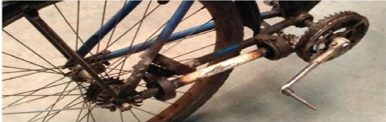
Figure 4.4- Bevel Gear Mechanism
