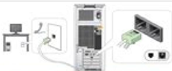
If you have a modem, connect a telephone cable to either of the modem connectors.
