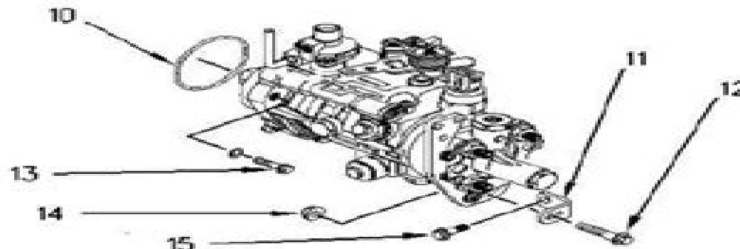
2. Install O-ring seal (10) on the fuel injection pump. Position the fuel injection pump on the front housing. Install bolts (13). Tighten the bolts to a torque of 25 N·m (18 lb ft).
