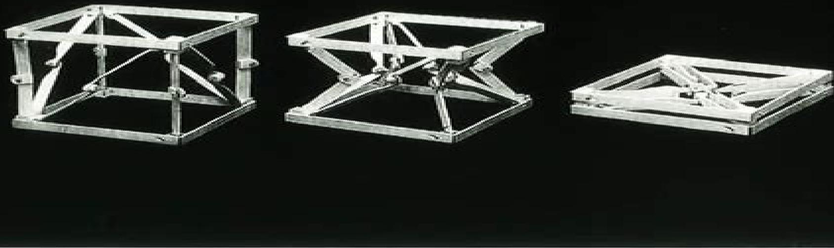
**Fig. 3.** Deployment sequence of NASA's STAC-BEAM geometry model.
