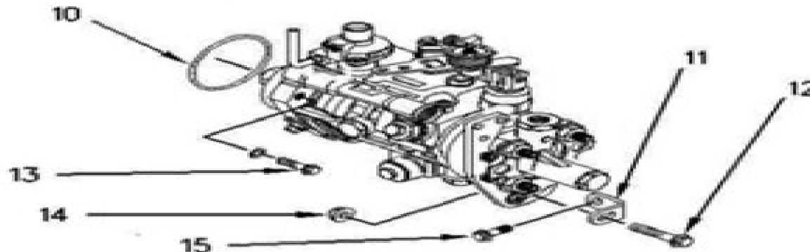
2. Install O-ring seal (10) on the fuel injection pump. Position the fuel injection pump on the front housing. Install bolts (13). Tighten the bolts to a torque of 25 N·m (18 lb ft).
