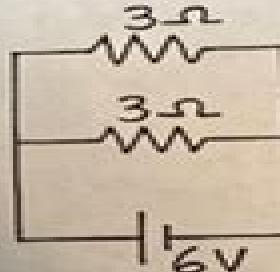
1. In the circuit shown to the left there is a voltage drop of 6 V across each 3- $\Omega$  lamp. By Ohm's law, the current in each lamp is \_\_\_\_ A. The current through the battery is the sum of the currents in the lamps. \_\_\_\_ A.
