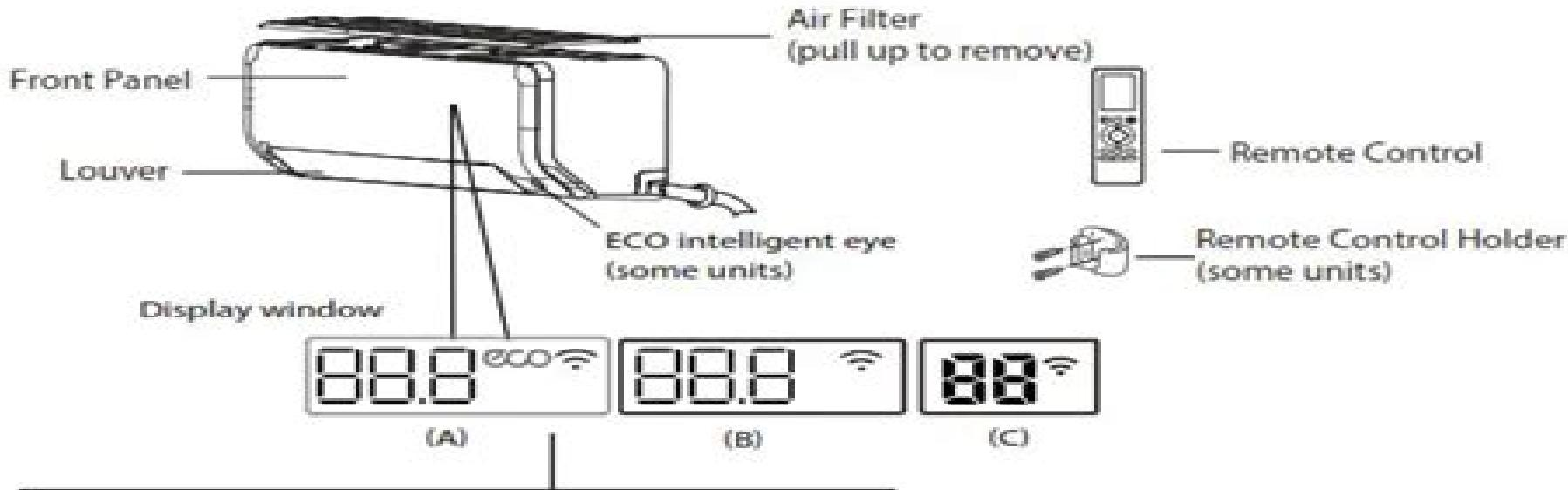
**88.8 88** Displays temperature, operation feature and error codes:
