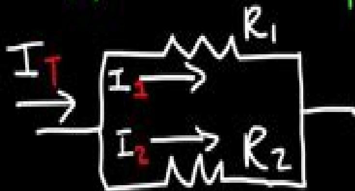
$$I_2 = I_1 \left( \frac{R_1}{R_1 + R_2} \right)$$
