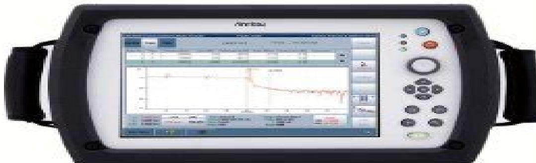
The compact size of the OTDR Application module allows another module (such as an additional OTDR or Gigabit Ethernet) to be inserted into a small bay adapter and up to three more into a medium bay adapter.
