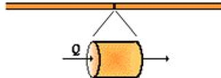
Current is the rate at which charge passes by a point on the circuit. If a small cross section of a wire could be isolated and the quantity of charge (Q) passing through this cross section in a certain amount of time (t) could be measured, then the current would be the  $Q/t$  ratio.
