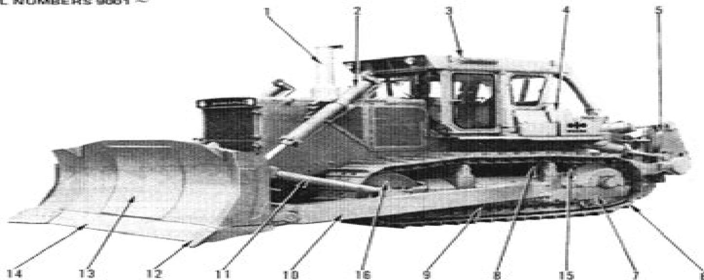
Note: The above picture shows a machine installed with a ROPS cab.
