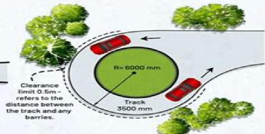
Turning circle refers to the space needed for a car to move in a circular track to ensure traffic control.
