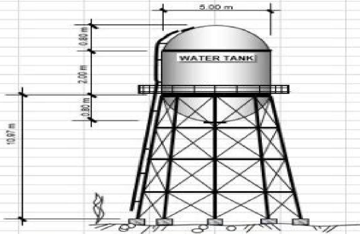
Water Tank Capacity = 360 U.S. Gallons
