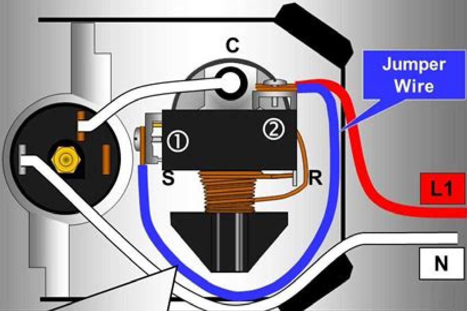
Remove jumper wire when installing start capacitor
