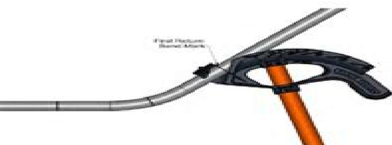
8. Keeping the bender and conduit together, flip the two parts upside down and put the bender's handle hilt on the floor, balancing the conduit in the air, allow the conduit to rotate 180° in the cradle. Slide the conduit down so the first bend is moving away from the bender head, aligning the **1<sup>st</sup> return bend mark** with the **Arrow Symbol** (See Stub-Up section, note 5).
