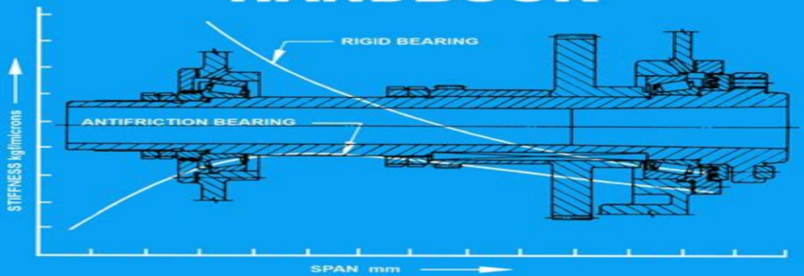
$$S = \frac{P}{\delta_1 + \delta_2} = \left\{ \frac{a^3}{3EI_L} \left[ \frac{L}{a} + \frac{L_a}{I_a} \right] + \frac{1}{S_A} \left[ \left( 1 + \frac{a}{L} \right)^2 + \left( \frac{a}{L} \right)^2 \frac{S_A}{S} \right] \right\}^{-1}$$
