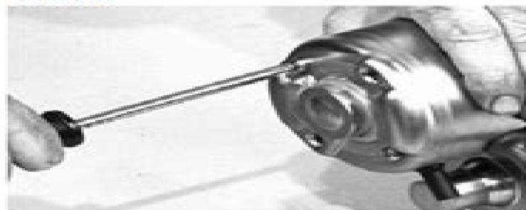
Install and tighten the screws that hold the brush holder.
