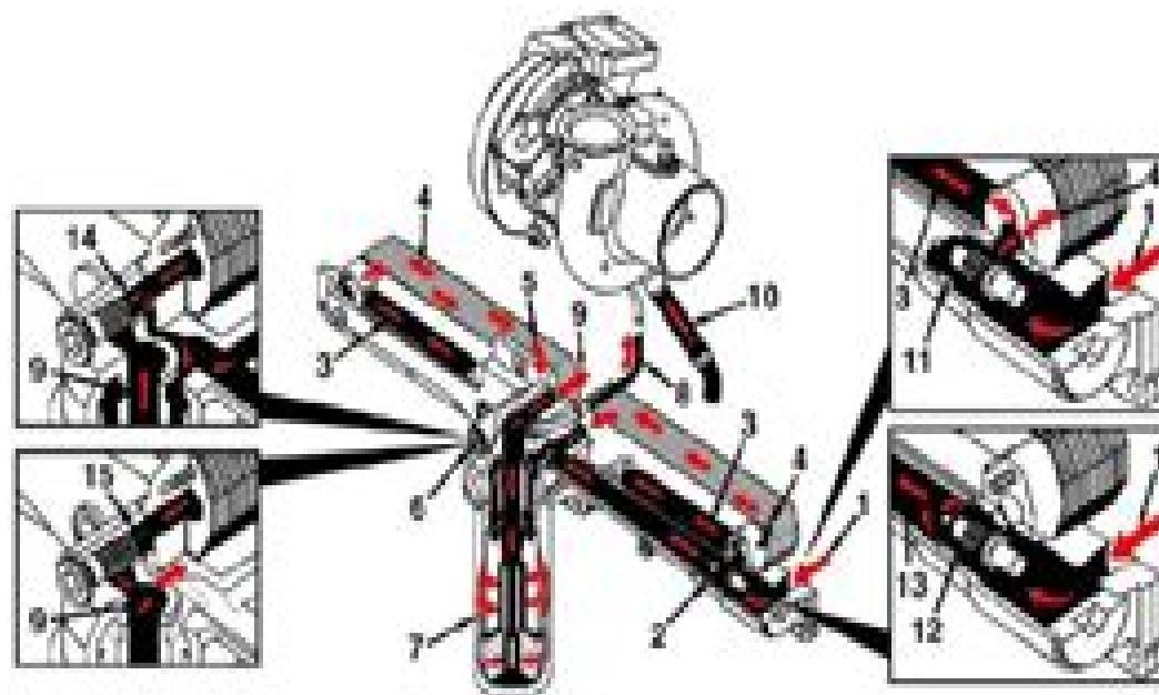
1. Lubricating Oil Flow from Oil Pump
