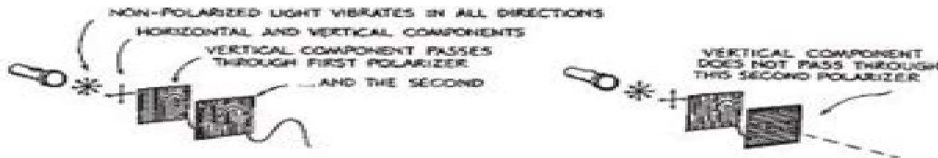
a. Light is transmitted by a pair of polarizing filters when their axes are (aligned) (crossed at right angles) and light is blocked when their axes are (aligned) (crossed at right angles).
