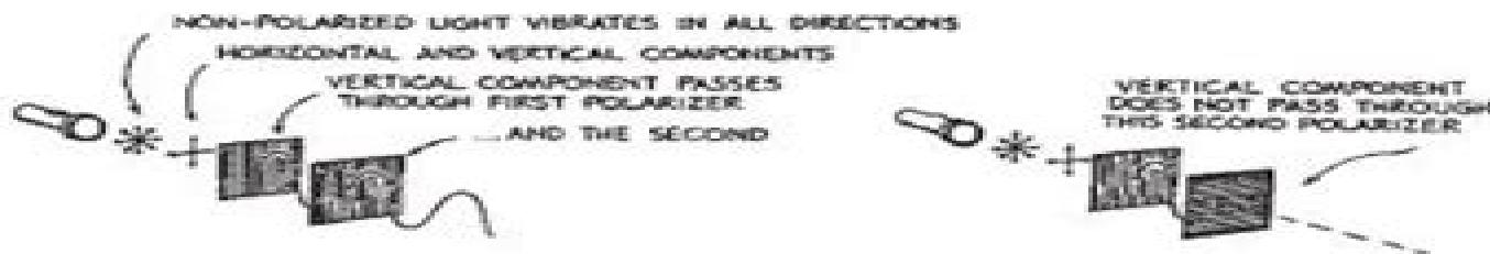
a. Light is transmitted by a pair of polarizing filters when their axes are (aligned) (crossed at right angles) and light is blocked when their axes are (aligned) (crossed at right angles).
